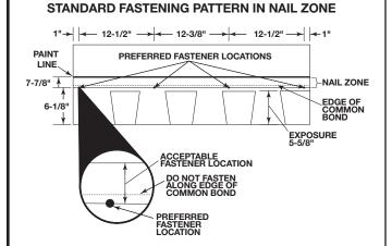
**3)** Mansard Fastening Pattern. (For use on decks with slopes greater than 21 in. per foot.) One fastener 1 in. from each end, one fastener 8-1/2 in. from each end and one fastener 16 in. from each end for a total of 6 fasteners per shingle. (See Mansard and High Wind Fastening Pattern illustrated below.)
