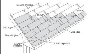
Second and Succeeding Courses: Remove 10-3/8 in. from the rake end of the first shingle in the second course, and continue with full width shingles for the remainder of the course, placing the top edge of each new shingle against the butt edge of the old shingle in the course above. This method should create an exposure of 5-5/8 in. after the first course. When beginning the succeeding courses continue to follow the Heritage application instructions. (See section 5).
