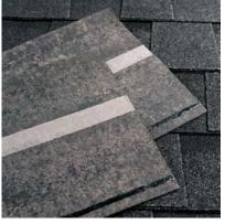
Titan  $XT^{\text{TM}}$  shingles feature a reinforcing strip of polyester fabric on the back of the shingle to provide added anchoring for the expanded nailing zone.
