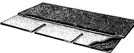
3-tab shingles are made with a single layer of fiberglass mat.
