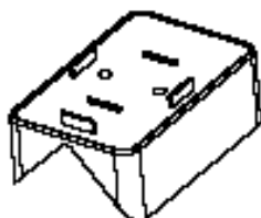
Lower Rail 45° PVC Bracket
