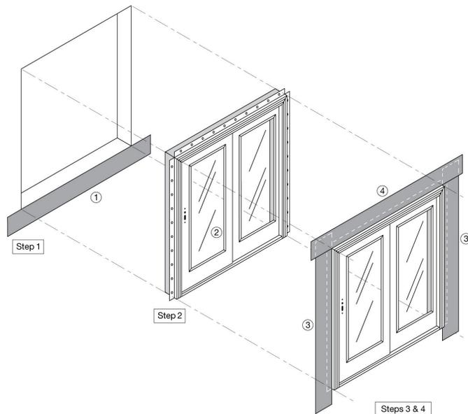
**Figure 3: Door installation detail for doors with integral flanges and flashing installed prior to WRB**
