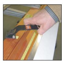
The raised tab on the Gauge makes a convenient place to hook a Tape Measure for layout. The tab is positioned to match the nose of the Anvil or the bend point of the workpiece.
