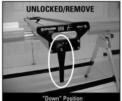
When the handle is in the "down" position, the Boom can be put on or taken off of the table.
