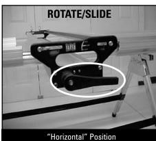
When the handle is in the "horizontal" position, the Boom can move freely while still attached to the saw table base.
