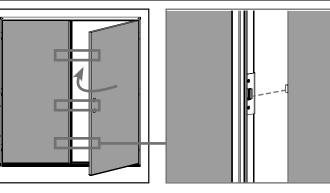
**b.** Close the active door panel and engage the lock to ensure the upper, middle and lower strike locations are properly engaged.
