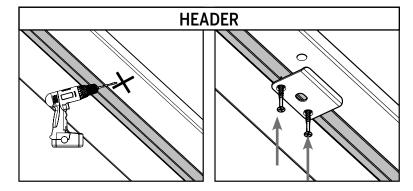
**c.** At the marked location on the header, drill a hole **3/8**" **in diameter** and at least **1-3/8**" **deep.** Install one of the strike plates into the header, using two  $#8 \times 3$ " screws.
