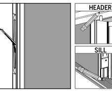
**b.** Engage the flip lever so the upper and lower bolt pins come in contact with the header and the sill. Mark these points of contact.
