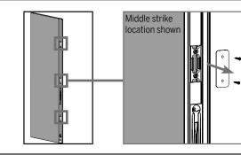
**a.** Remove the upper, middle and lower dummy strike plates.
