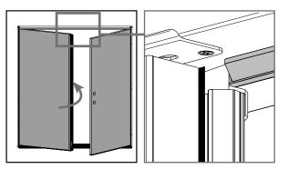
**c.** Close the inactive door panel. Ensure the weatherstrip forms a secure seal around the trim cap.
