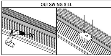
**d.** At the marked location on the sill, drill a hole **5/8" in diameter** and at least **1-3/8" deep.** Install the other strike plate into the sill, using two  $#8 \times 3"$  screws.
