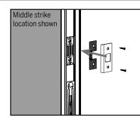
Cut Here **b.** At each location install new strike plates by screwing into the retainers.
