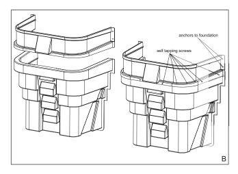
All Wellcraft wells are designed to Meet IRC 2003 International Residential Code requirements, Section 310, for Emergency Escape/Rescue window opening for one and two family dwellings. The 2060 well is designed to be used with up to a 4 foot side sliding window that meets the egress code. 10-year limited warranty on window wells in effect when installation instructions are followed. Contact Wellcraft. Inc. for details.
