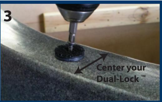
3. Using the provided self-tapping screws attach all the hardware for your cover. Be certain to attach the Dual-Lock™ in the center of the well wall.
