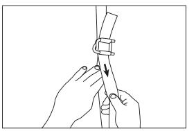
8 Brace strap and pull tail to cinch loop and to remove any excess slack.
