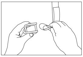
1 Feed strap under load before threading buckle. Fold tail of strap and form loop. Hold buckle with legs on top and pointing right.
